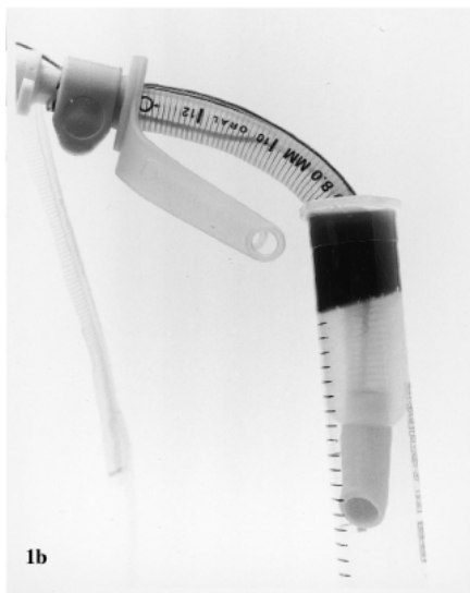
FIGURE 1: Tracheostomy tube cuffs inflated in a 2cm diameter rigid cylinder to represent the trachea. Dye was instilled above the (a) Shiley and (b) Silicone cuffs to observe leakage in vitro.
